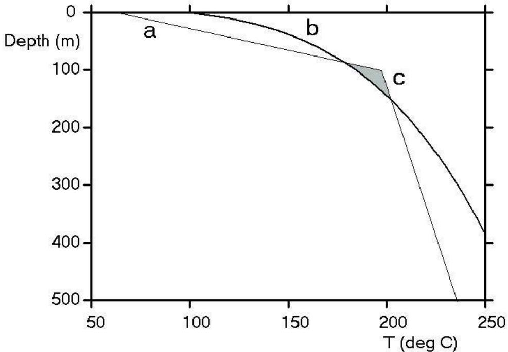
Figure 2. (a) Idealized profile of well temperature following stimulation. (b) The temperature-pressure characteristic of equation (1b). (c) Overlapping region in which wet steam is formed.
