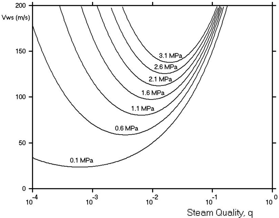
Figure 1. Speed of Sound,  $v_{ws}$ , as a function of pressure and quality,  $q$ .
