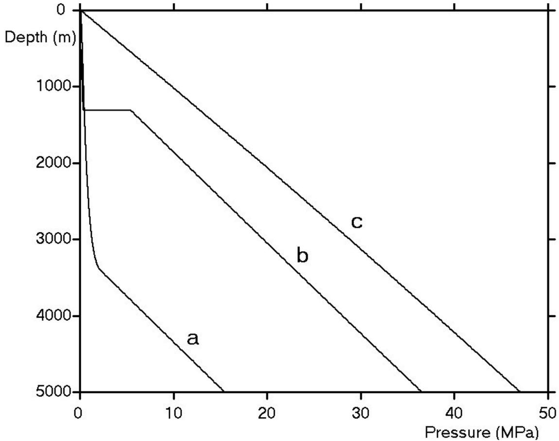
Figure 3. Pressure as function of depth. (a) Production well without valve. (b) Production well with pressure release valve. (c) Injection well.
